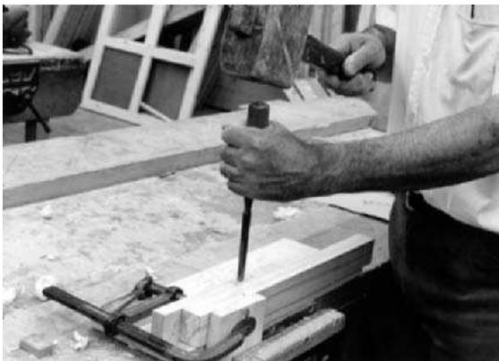
**Fig 5.64** Chopping a mortice hole – notice the use of scrap wood to protect the bench and work piece, and how the clamp has been laid flat with protruding bar and handle positioned towards the well of the bench, out of harms way
