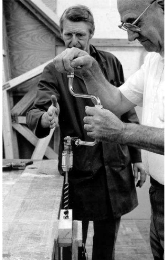
**Fig 5.55** Aligning a bit for vertical boring using hand signal guidance from an assistant taking the second vertical viewpoint
