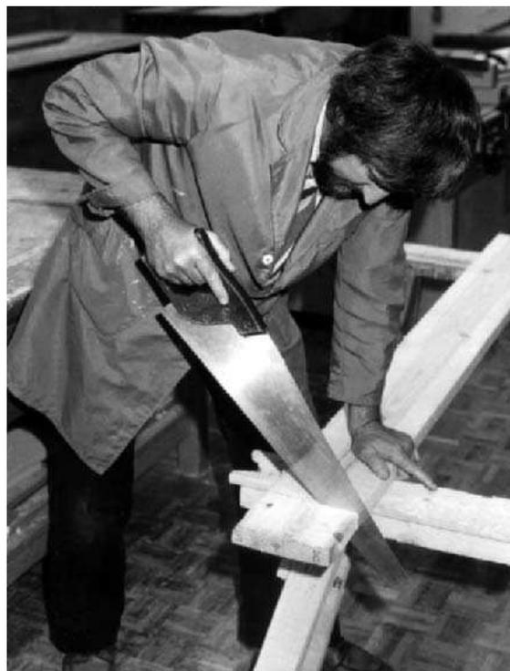
**Fig 5.14** Cross cutting with a hand saw (notice the position of the fore finger and how the arm and shoulder is in line with the saw blade)
