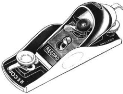
**Fig 5.30** Block plane (with kind permission from Record tools limited)
