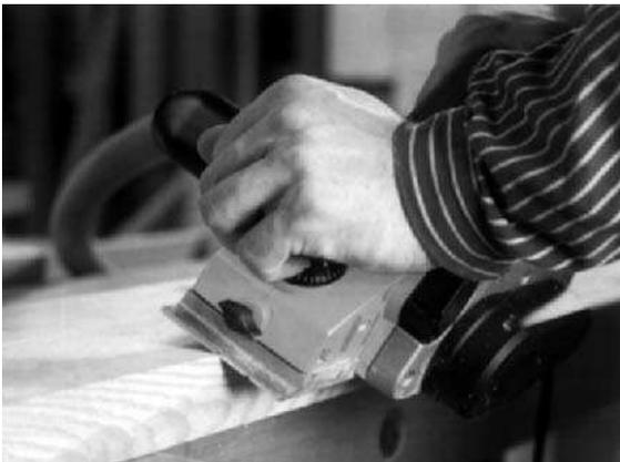
Cutting a chamfer by using the middle 'V' groove in the sole as a guide
