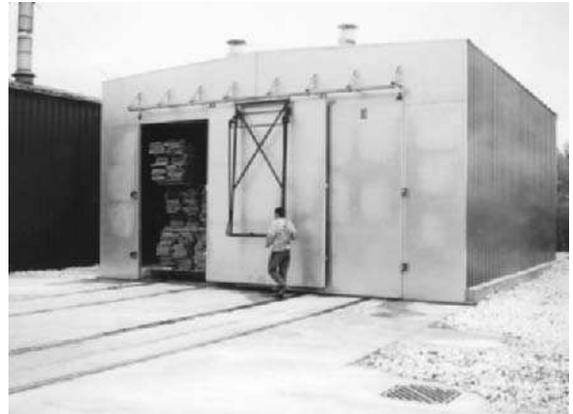
**Fig 1.45** External sited compartment dryers (with kind permission of 'Kiln Services Ltd')
