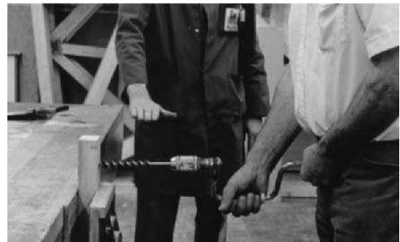
**Fig 5.56** Aligning a bit for horizontal boring using hand signal guidance from an assistant taking the second horizontal viewpoint
