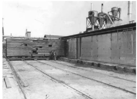
**Fig 1.46** Externally sited battery of compartment dryers – one being loaded with timber (with kind promise of 'Wells Ltd')
