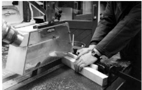
(c) Cross-cutting a compound angle by tilting the saw blade and using an angled cross-cutting fence and sliding (rolling) table. Notice change of saw guard to accommodate the tilted blade.
