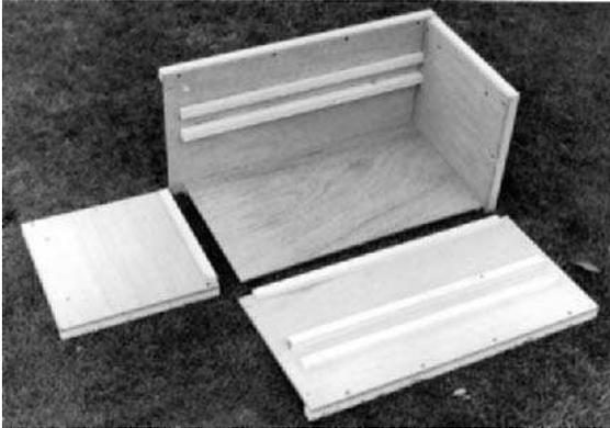
**Fig 11** Porterchest sides and base assembly
