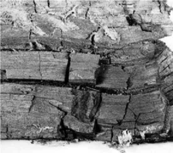
**Fig 2.8** Dry-rot damage showing the cuboidal effect (with kind permission of Rentokil)
