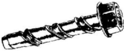
**Fig 12.28** Screw bolt
