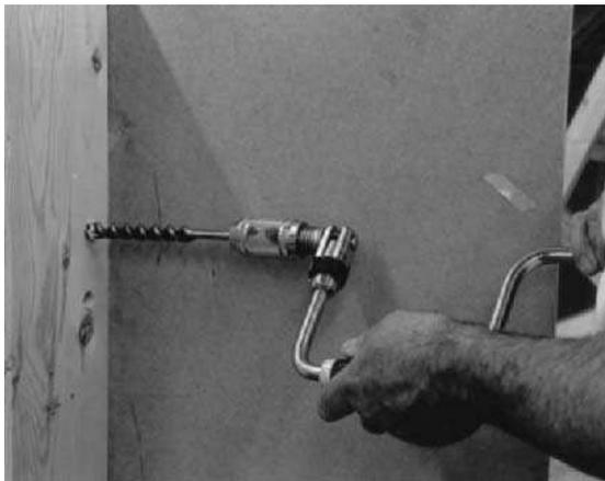
**Fig 5.54** Using the ratchet mechanism of a carpenter's brace when full sweep is restricted
