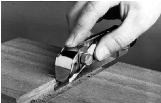
**Fig 5.35** Side rebate plane in the use (with kind permission from Stanley tools limited)
