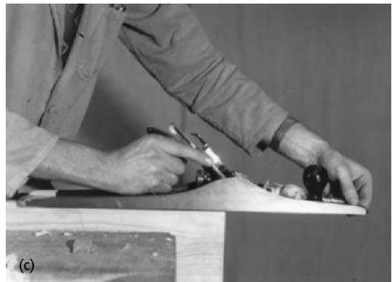
**Fig 5.43** Using a try plane (jointer)
