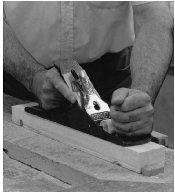
**Fig 5.40** Flattening – planing the face of a piece of timber placed against a bench stop
