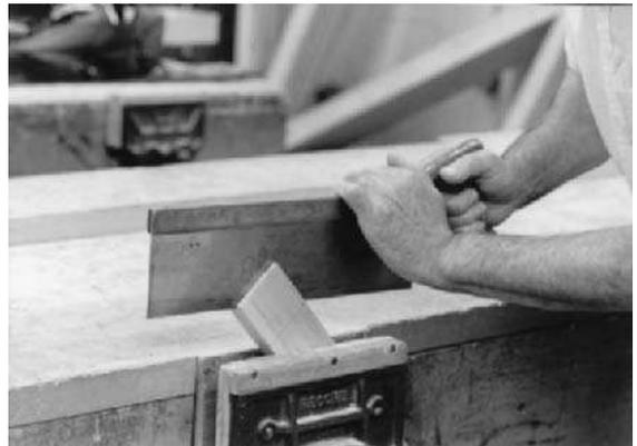
**Fig 5.18** Sawing down the grain with a tenon saw
