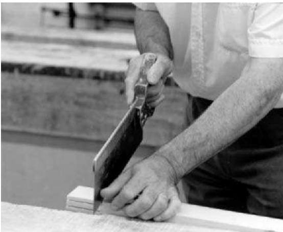
**Fig 5.17a** Tenon saw – starting a cut, vice held
