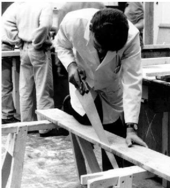
**Fig 5.13** Ripping with a hand saw (notice the position of the fore finger and how the arm and shoulder is in line with the saw blade)
