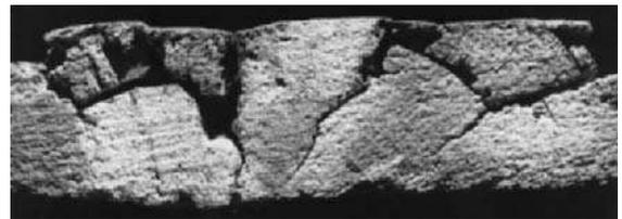
**Fig 2.11** Wet-rot damage to end grain – (with kind permission of Rentokil)
