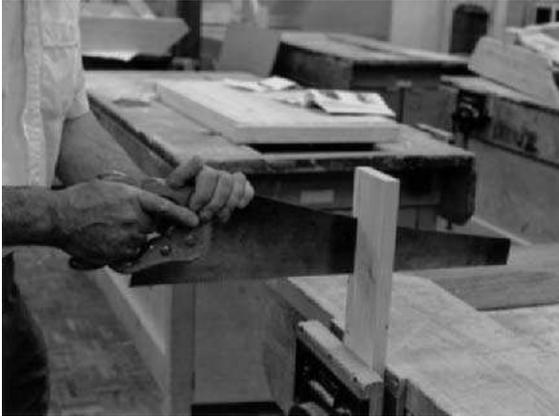
**Fig 5.15** Sawing down the grain (vertically) with a panel saw
