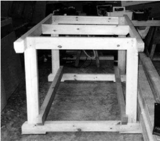
**Fig 20** End frames, base runners, top facings and cross bearer
