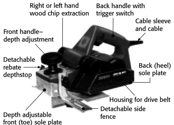
**Fig 6.39** Portable powered planer
