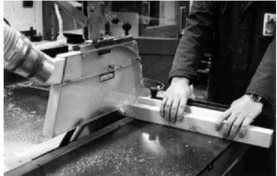
(a) Cross-cutting square by using the cross-cutting fence and sliding (rolling) table.
