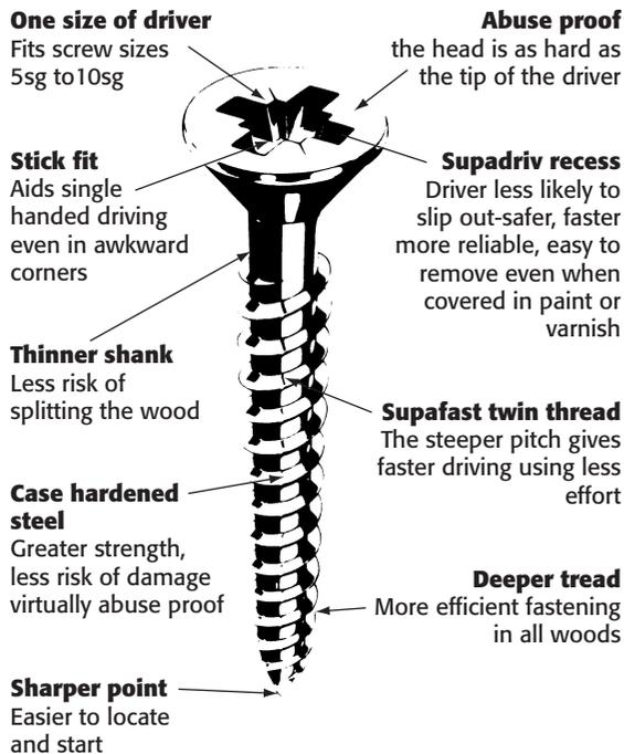
**Fig 12.6** Supafast threaded screws
