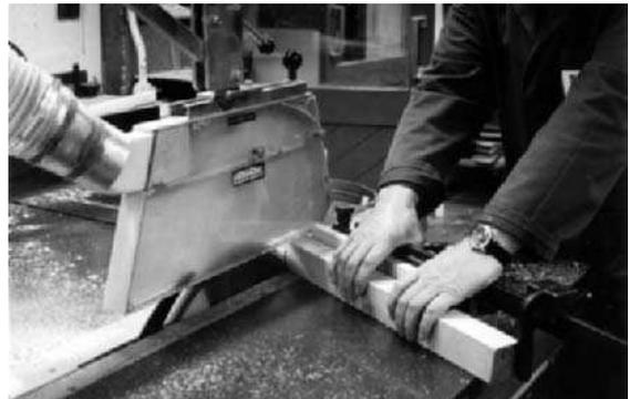
(b) Cross-cutting at an angle by using an angled cross-cutting fence and sliding (rolling) table.
