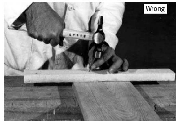
**Fig 5.69** Holding a hammer
