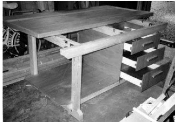
**Fig 21** Bench carcase, drawer unit and shelf
