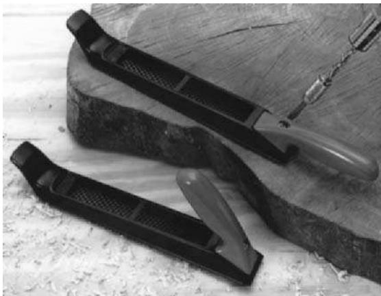
**Fig 5.66** Selection of Stanley 'surform' tools (with kind permission from Stanley tools limited)
