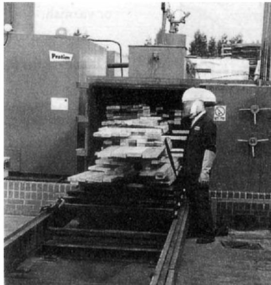
**Fig 3.5** 'Protim' double vacuum treatment plant (courtesy of Protim Ltd)
