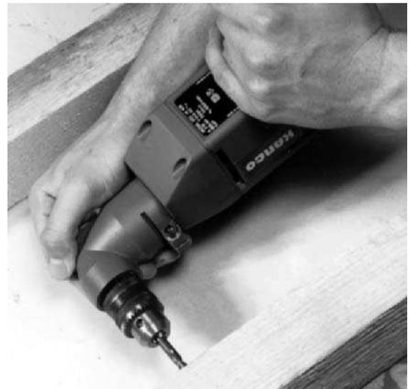
(b) Using an angle-drill attachment
