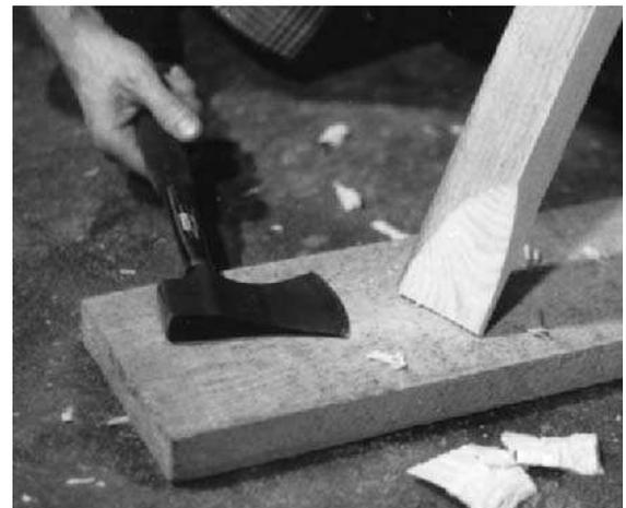
**Fig 5.65** Using an axe to cut a tapered end on a short length of timber
