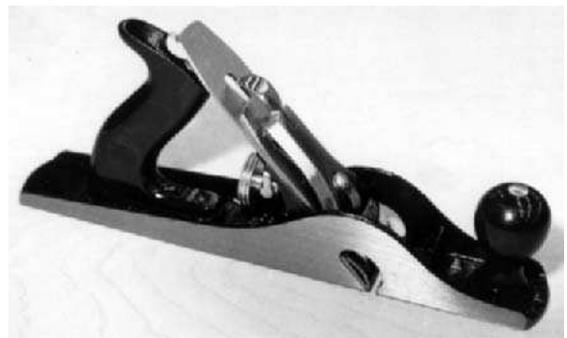
**Fig 5.28** Bench rebate plane (carriage or badger plane) (with kind permission from Stanley tools limited)
