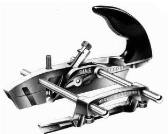
**Fig 5.36** Plough plane (with kind permission from Record tools limited)
